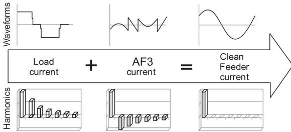
In the following example first figure shows the recorded input current waveform of a six pulse thyristorised rectifier.
